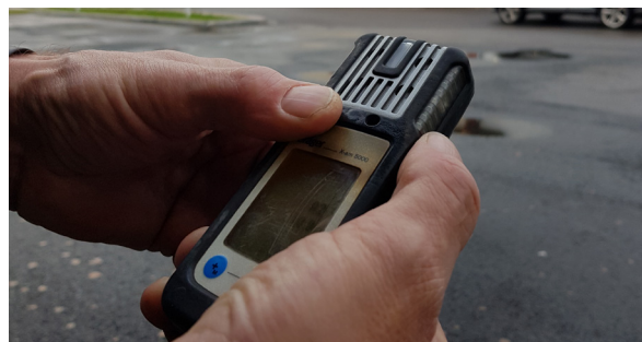
Gas measuring instrument. Image: Drammen Regional Fire Service IKS.
