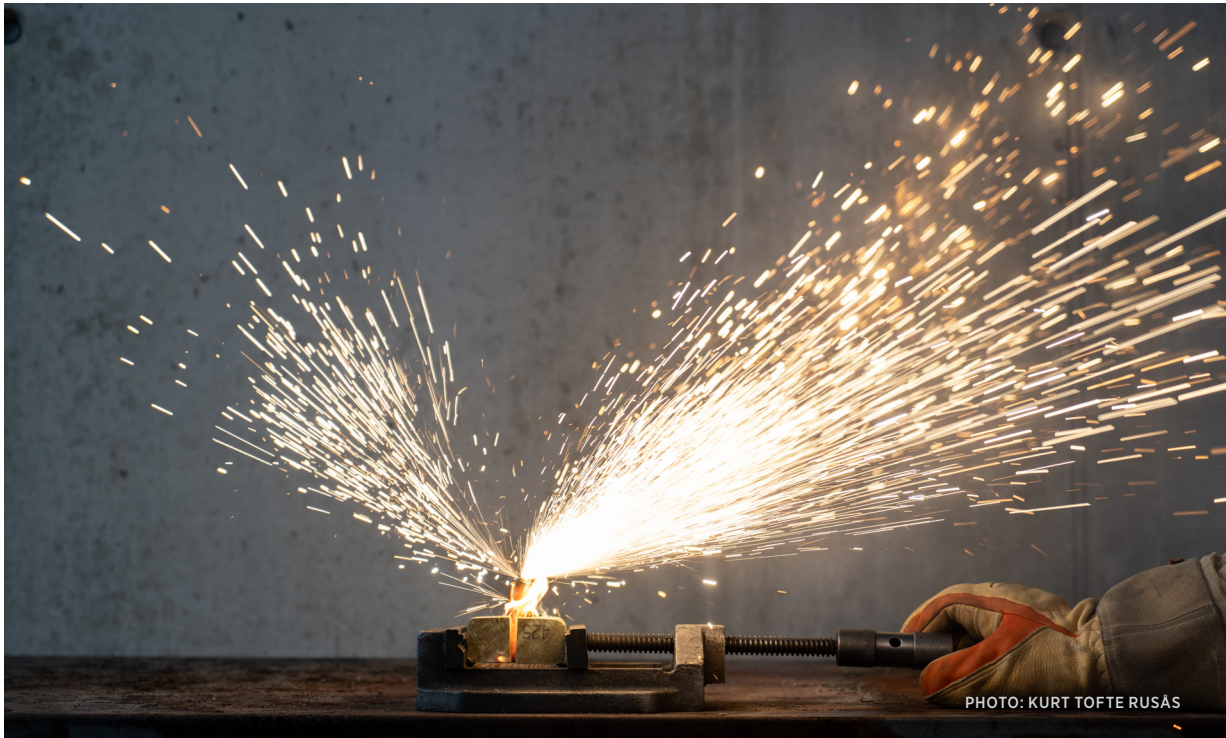
Experiment in which battery cells are subject to mechanical influence, leading to puncture and jet flames.
