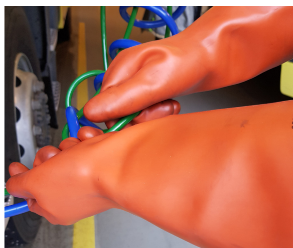
1000-volt gloves. Image: Drammen Regional Fire Service IKS.
