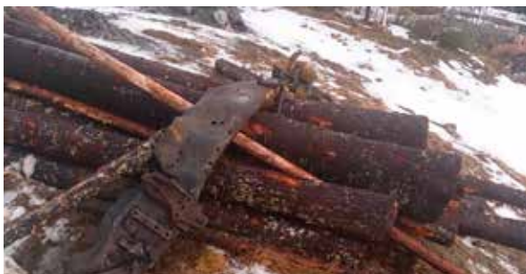
FIGURE 28. Fragment that illustrates deformation of steel due to heating.
