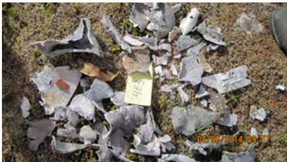
FIGURE 20. Small aluminum fragments found at approximately 150 meter in easterly direction.
