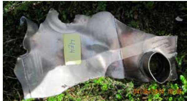
FIGURE 25. Fragment from the production diesel tank.
