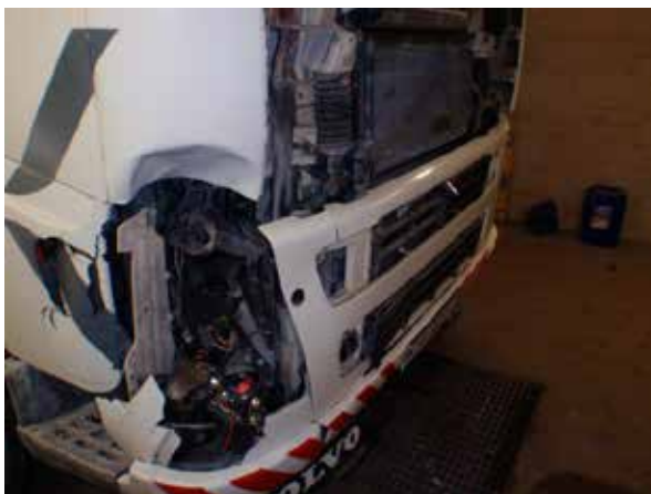
FIGURE 4. Picture of damages on MEMU F-114 after collision with the elks.
