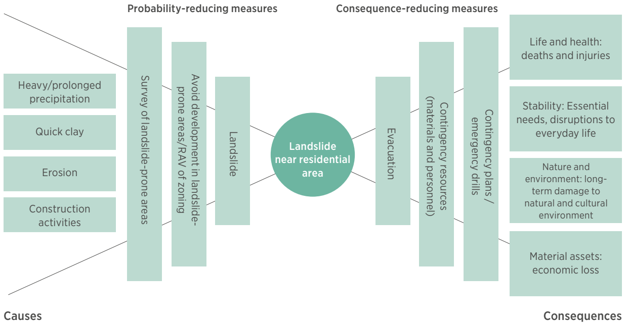
FIGURE 2. Example of a bowtie diagram based on the hazard “landslide near residential area”.
